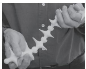
Object with 7 articulating joints from a 3-D printer. Courtesy of MIT Media Lab.
