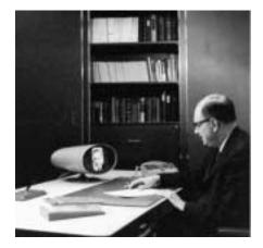
Figure 4. A landmark in the development of Teleconferencing was when Bell Labs introduced the Picturephone at the World Expo in 1964; the world's first interactive video-enabled telephone. Original Caption by Science Service © Bell Telephone Laboratories
