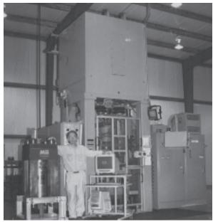
Computer-driven, powder metallurgy press (foreground) with traditional press behind. Courtesy of Mii Technology.
